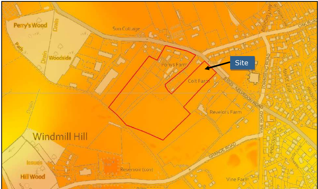
Figure 2: Filtered LIDAR survey data at 1m resolution where higher ground is denoted by red and orange colours and lower ground is denoted by yellow and green colours
